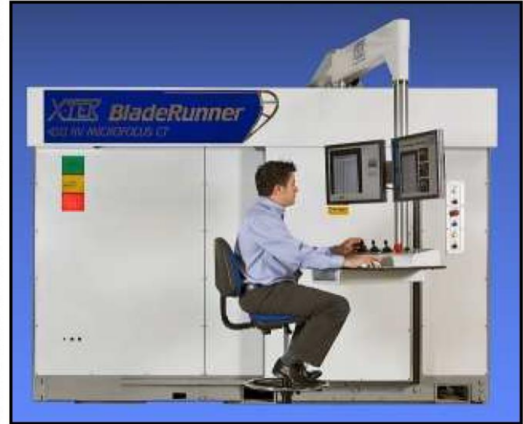
Figure 2. X-Tek's Bladerunner 450kV microfocus X-ray CT system
