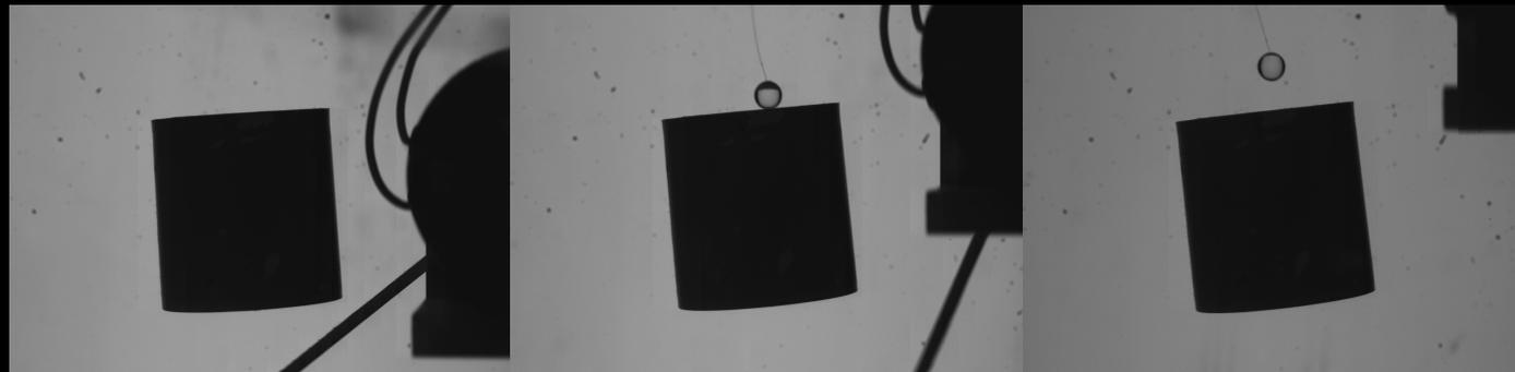
$v_{\text{imp}} = 1.42 \text{ m/s}$ , Target: 50 % porosity
