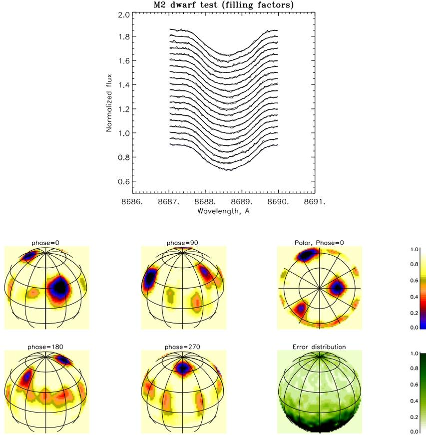
**Fig. 2.** Test inversion from an artificial M2 star ( $T_{\text{eff}} = 3500$  K,  $\log g = 5.0$ ) using “filling factor” as the inversion parameter. One atomic line (Fe I 868.862 nm) and many molecular lines, mostly CN, were used. Thin lines in the top panel are the artificial data, the thick lines are the reconstruction with object’s principal components. The lower panels show the reconstructed image.
